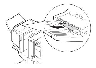
**2.** Operate the Finisher lever (1) and move the Finisher away from the Inverter.
