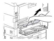
**4.** Put the paper guide back into position and close Tray 1 side cover.
