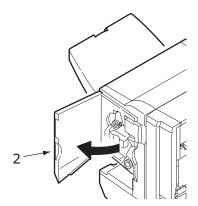
**3.** Continue to turn the lower knob (3) clockwise until any jammed paper is completely ejected.
