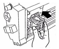
**11.** Ensure that the staple cartridge is securely installed back into the staple unit then push the staple unit fully home.
