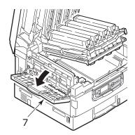
**8.** Open the side cover (paper exit) (8) and remove the jammed paper.
